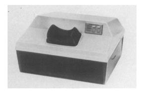
Ultra-Violet Products, Inc., is marketing its new UVP Color Matching Cabinet as a fast, simple color matching tool, specially designed to aid in visual identification of potential color mismatches. The color samples are first examined under a daylight lamp, then under a pink UVP matching lamp. If the match persists, the firm says, the two colors will always match to all viewers under all conditions. Information: UVP Inc., 5100 Walnut Grove Ave., San Gabriel, CA 91778 (tele: 213-285-3123).
