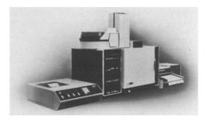
Varian has introduced its Model 3711 Automatic Gas Chromatograph which automates the gas chromatography process from injection and separation through peak measurement, calculations, and final report. Model 3711 is a two-unit instrument consisting of controller and dualcolumn chromatography. Information: Bill Ballandyne, Varian Associates, Instrument Division, 611 Hansen Way, Palo Alto, CA 94303 (tele: 415-493-4000).
